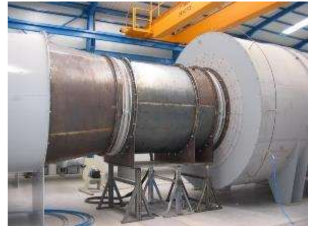
High temperature fan testing according to standard EN 12.101-3
