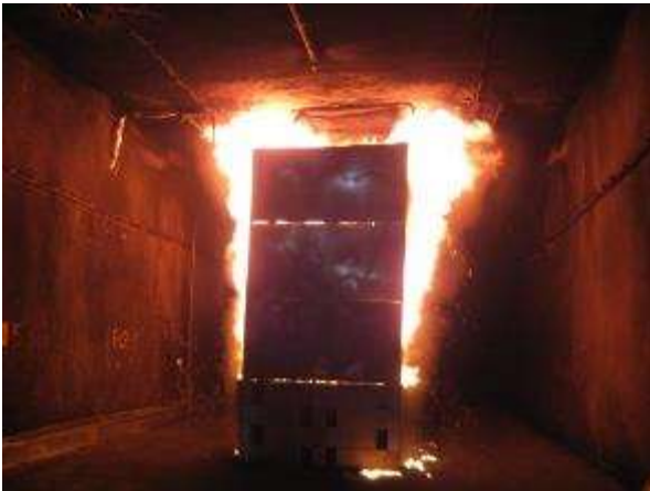
Full scale tunnel fire and ventilation tests
